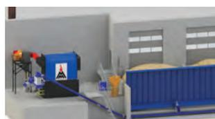
Messersmith Manufacturing provides design, fabrication, installation, and startup of biomass boiler systems with thermal outputs ranging from 600 kW to 6 MW. The systems can use fire-tube or water-tube boilers, providing hot water or high-pressure steam for electricity generation. A fixed, sloping grate system combines with preheated combustion air to provide clean, efficient combustion with less than
