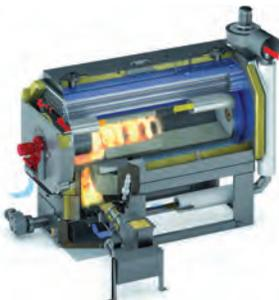
Fink Machine is an authorized sales and service agent for Viessmann-KOB commercial boilers from Austria. The Pyrot and Pyrotec lines range from 100 kW to 1.25 MW thermal, offer 4:1 turndown ratios, and use both wood pellets and wood chips with 50% moisture content with a thermal efficiency of 90%. Recirculation flue gas technology, lambda (oxygen) sensors, temperature sensors, and walking floors
